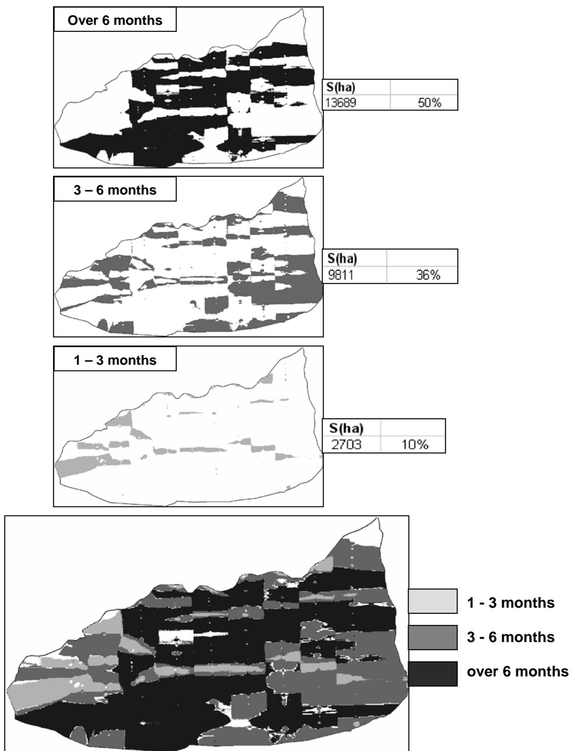
Figure 4: Results of hydrological scenarios showing the hydro period map of Pardina area after re-flooding.
