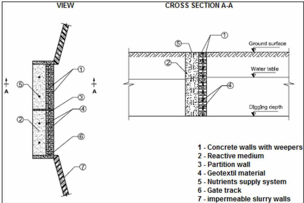
Figure 3: The construction scheme - solution 1.
