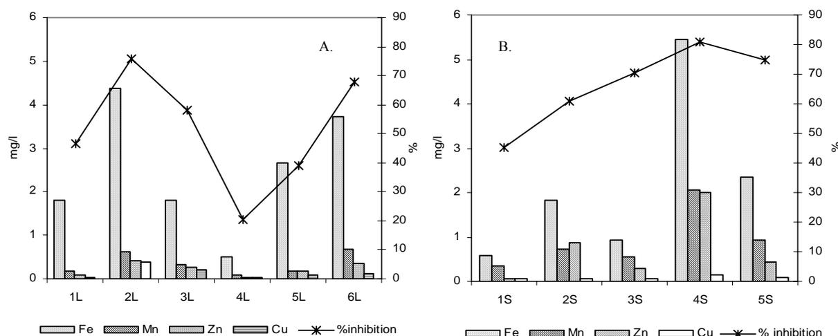
Figure 1: The bioluminescence inhibition (%) distribution and heavy metal concentrations in Lăpuș (A) and Săsar (B); 1L to 6L - sampling sites on Lăpuș; 1L - upstream Băiuț; 2L - downstream Băiuț; 3L - Upstream Târgul Lăpuș; 4L - downstream Târgul Lăpuș; 5L - upstream confluence Cavnice; 6L - downstream confluence Săsar; 1S to 5S - sampling sites on Săsar river; 1S - upstream Baia Sprie; 2S - downstream Baia Sprie; 3S - downstream Romplumb; 4S - downstream Cuprom; 5S - downstream Baia Mare.
