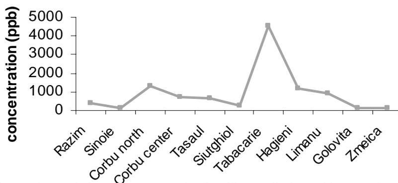
Figure 10: Total nitrogen concentration in effluents discharged in natural waters.
