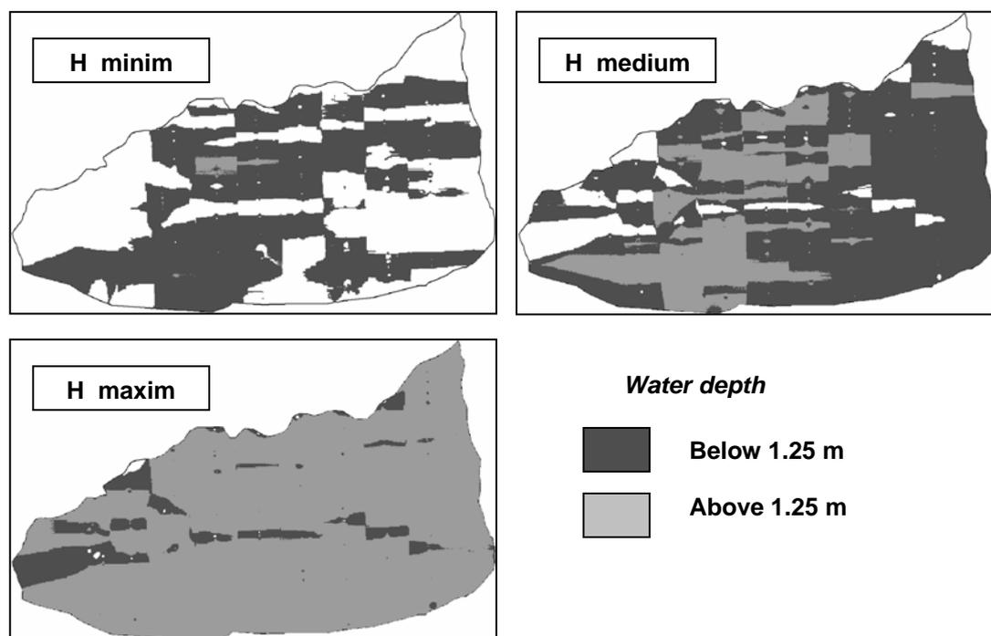
Figure 3: Flooded maps of Pardina area (below and above 1.25 m water depth) for different hydrological regimes of the Danube River.
